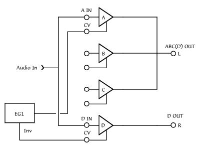
To fade between two inputs use the connection below. You can use A, B, or C.
