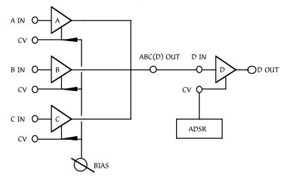
Another use for VCA "D" takes advantage of it's 10X gain. External signals from keyboards, etc. can be brought up to modular synth levels for use with the Final Filtre, Time Machine, Mini Wave, etc.
