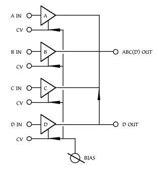
The arrows indicate the normalled connections. The Mix pot on each input is not shown.
